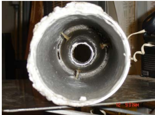
Figure WEA72-9: Shroud showing salt accumulation, with nozzle clear.
