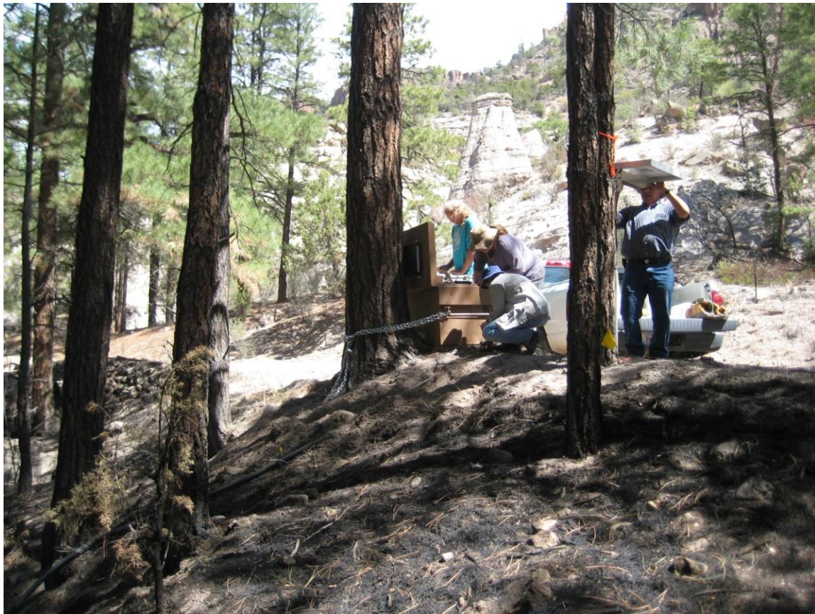
Figure LSW11-5. Bureau staff installed an ISCO water level monitor and stormwater sampler in Bland Canyon near Pueblo de Cochiti. (Note the “Tent Rocks” in background.)
