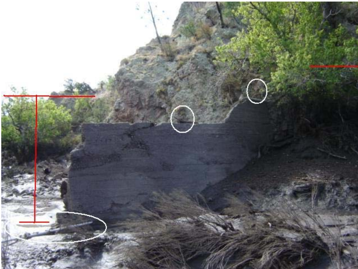
Figure LSW11-6. Bureau monitoring equipment was washed out at the sampling location at the old dam abutment in Peralta Canyon after a flash flood in August 2011. Damaged equipment is circled in the photo above: the sampler suction line (lower left); the solar panel (middle); and the sampler, battery and flow meter (upper right). The red line on the left marks the vertical height from stream channel to top of abutment where the sampler was located, 12 feet. The red line on the right marks the approximate height of storm flow, 15 feet.
