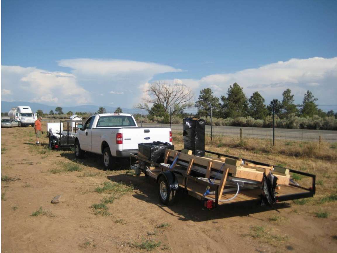
Figure LPL05-1. Bureau Scientist Bill Bartels installed the new solar-powered mobile air sampling unit at the Las Alamos Airport. The unit includes a trailer, sampler, and solar panels and replaces the older solar unit.
