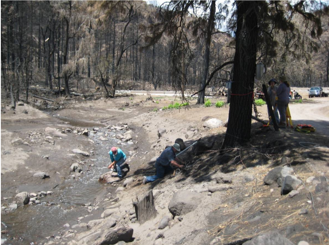
Figure LSW11-4. Bureau staff set up an ISCO water level monitor in a severely burned area of Cochiti Canyon just west of the Dixon Apple Orchard. Note the equipment fastened to the tree. All visible trees in this image were burned in the Las Conchas fire and were later felled (excluding the tree supporting Oversight Bureau equipment) by State Land Office work crews.
