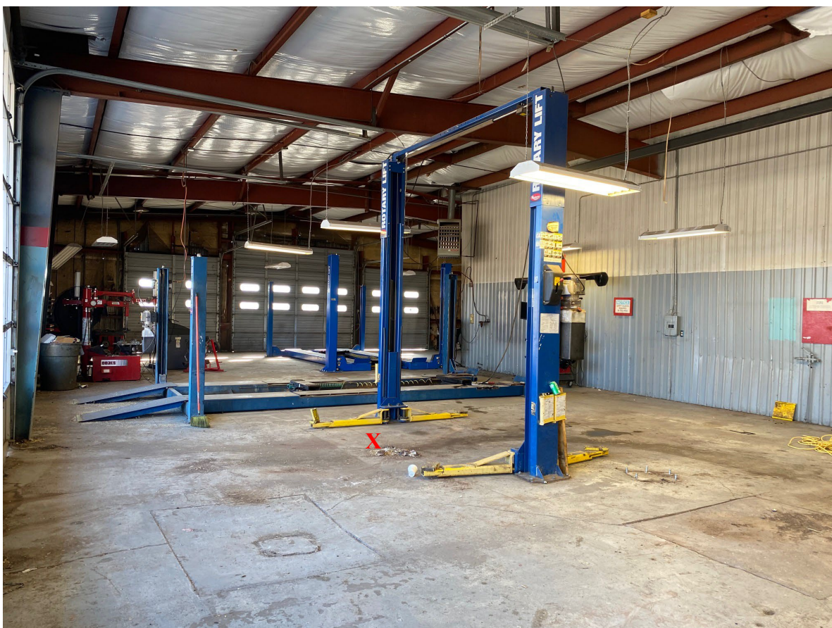
Figure 5. Photo of hydraulic lift S-2 prior to excavation. Lift cylinder is noted with X.
