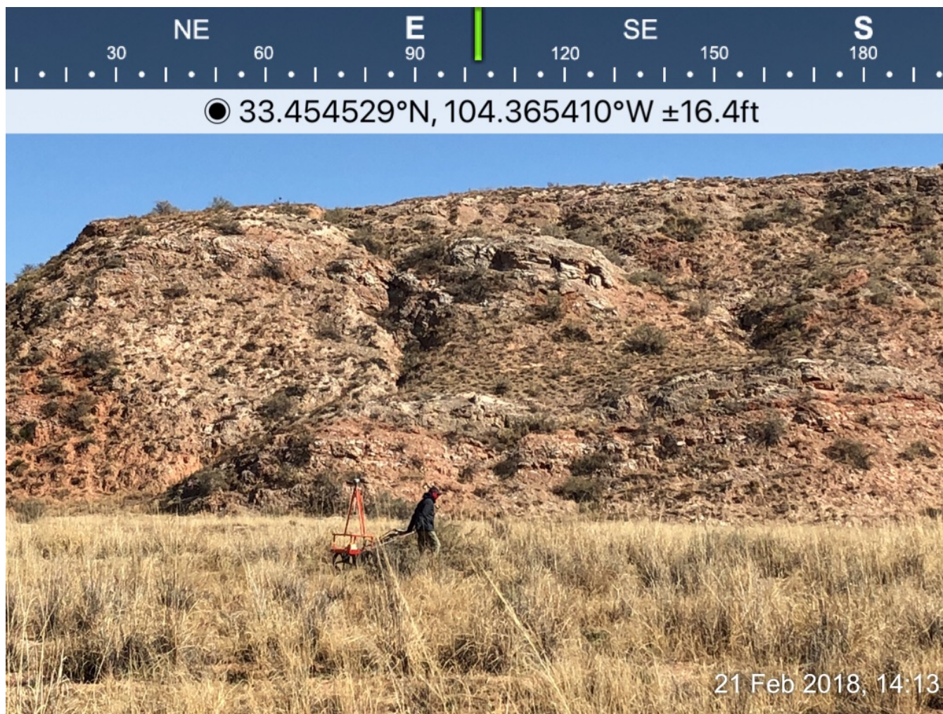
WESTON Geophysicist collecting DGM data using the Geonics EM61-MK2A metal detector at the Roswell North Range MRS during the RI.
