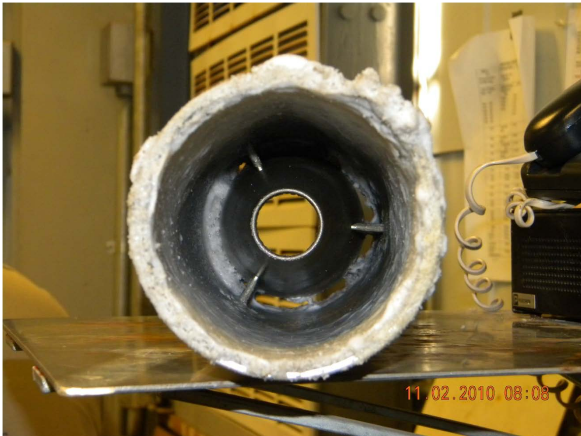
Figure WEA72-1: Probe pull of Station A, Skid A-1 on November 2, 2010. The shroud was occluded to a marginal status
