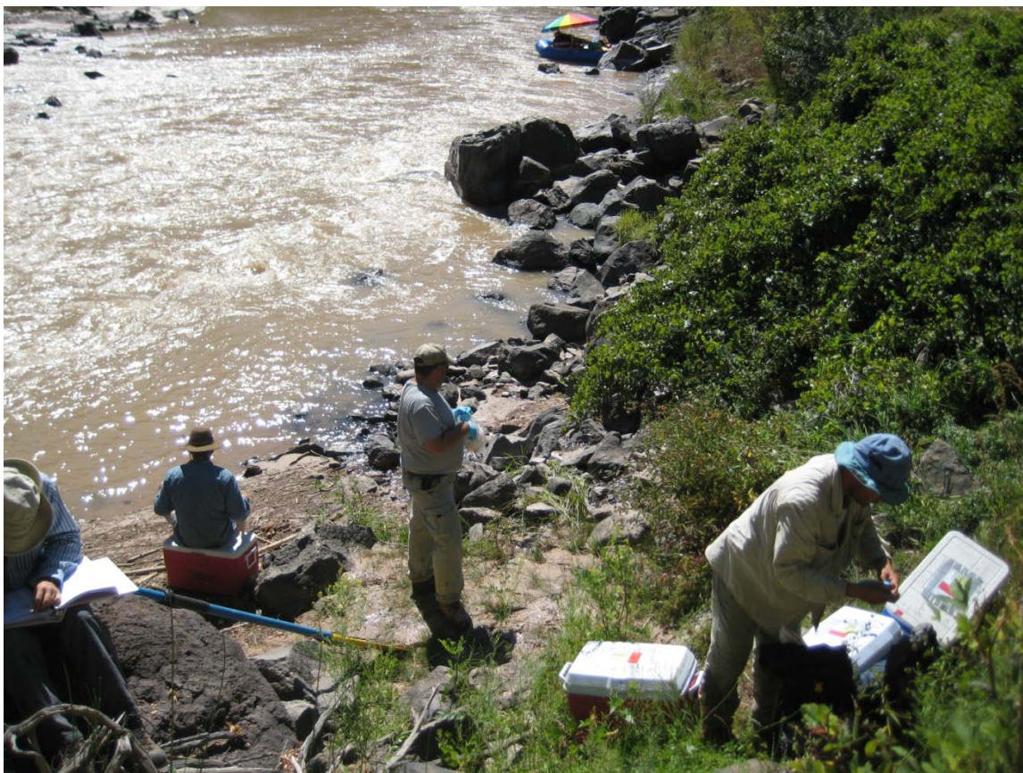
Figure LSM09-1: The White Rock Canyon springs sampling team prepares to sample Spring 6 in Ancho Canyon at the Rio Grande, Laboratory analyses will include tritium, high explosives, volatile organic compounds and chlorine-36 (a long-lived radionuclide).
