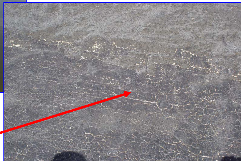
Right: EP2 liner showing effects of exposure to air and sun
